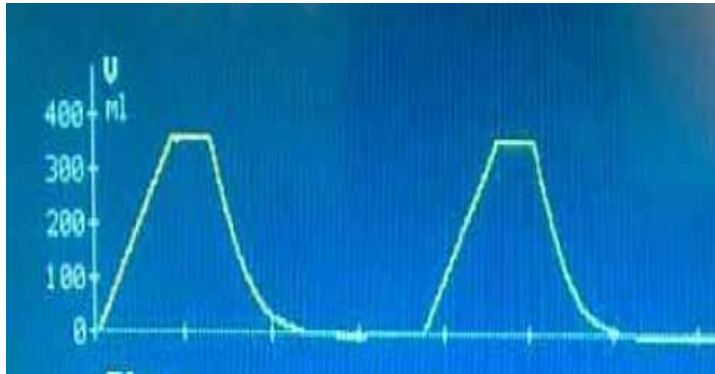
Figure 3 : Pressure vs time waveform during volume controlled mode (VC)
